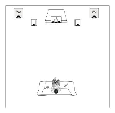
Note: Because of the massive motor structure used in the Evolution subwoofer driver, it is not possible to magnetically shield it. Make sure you place the subwoofer at least 18" from any television to avoid discoloration.
